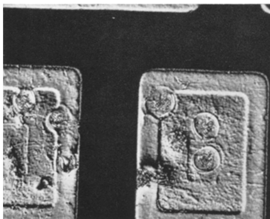
Figure 18 After modified Dash etch for 40 sec (X136).
