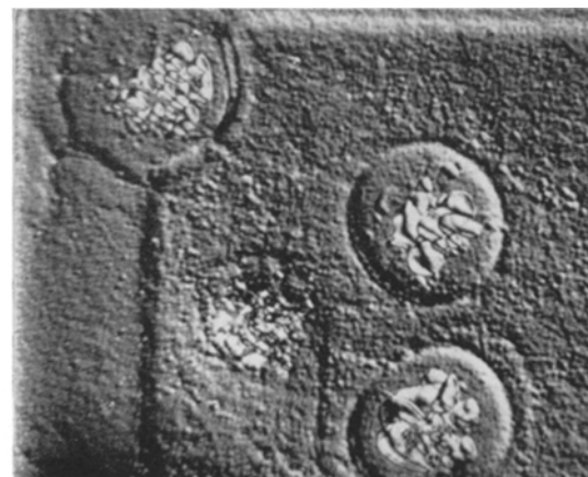
Figure 19 After modified Dash etch for further 40 sec (X360).
